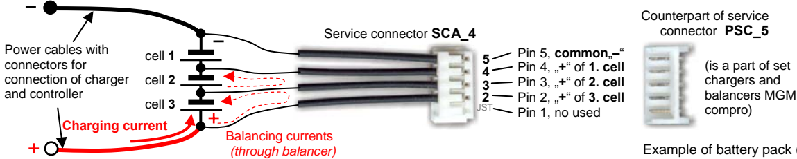
Example of battery pack (3 cells) with power wires, connectors MP JET and service connector SCA_4:
