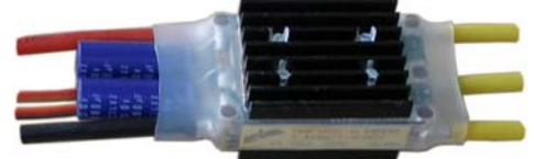
ESC with external heatsinks (38 mm)
