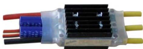
ESC with external heatsinks HC_02
